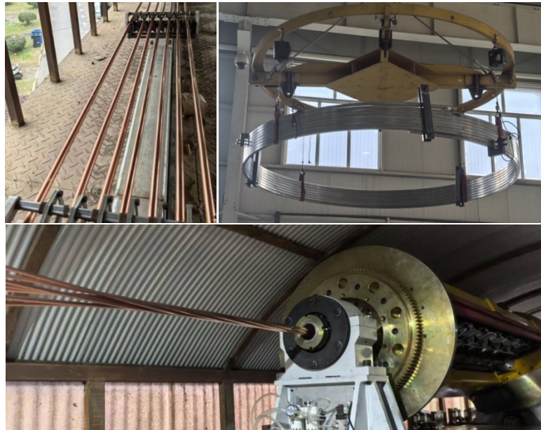
Fig. 3 Long length REBCO CICC manufacture
