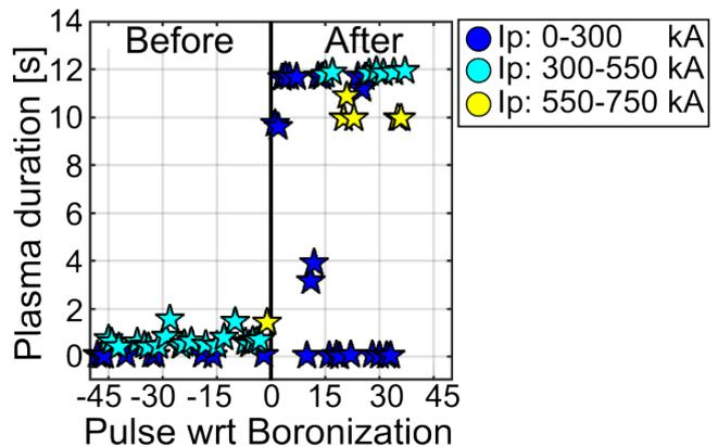
Figure 3: Plasma duration and current before and after GDB with bulk tungsten tiles and half of the injection points used.
