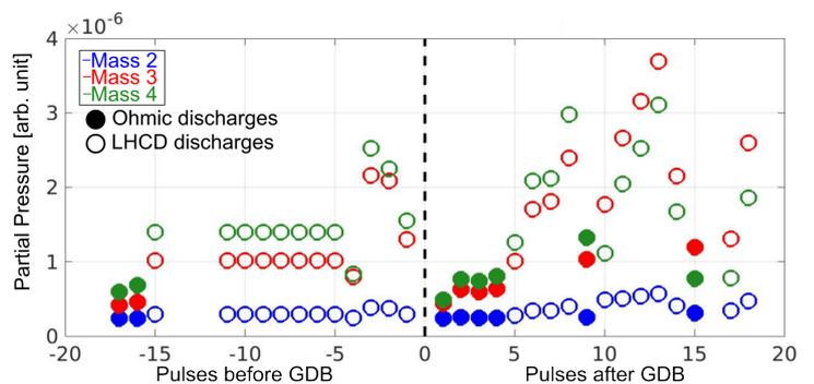
Figure 1: Partial pressure as derived from RGA measurements in the divertor exhaust gas before and after the GDB (vertical dashed line) for 3 different masses.
