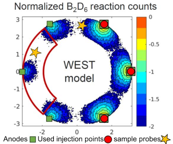
Figure 2: Top view of WEST showing toroidal position of glow anodes and diborane injection points usable during boronization. Colormap showing the diborane reaction rate from Monte Carlo tracing [4] of diborane in a glow discharge plasma background of WEST.
