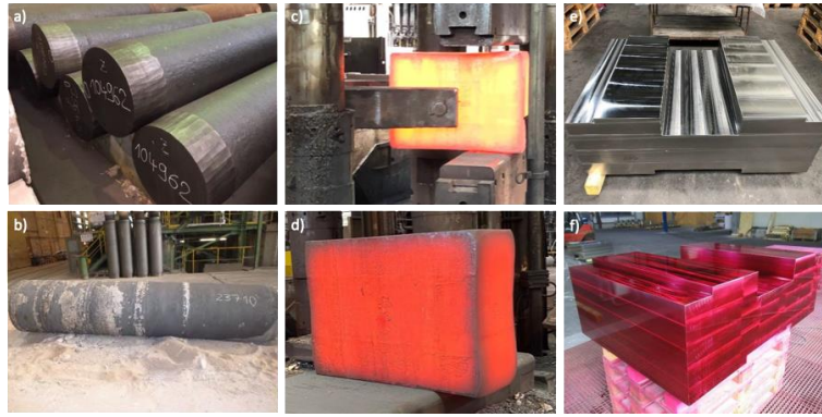
Fig. 1 Fabrication of the SS316L(N)-IG on each step
