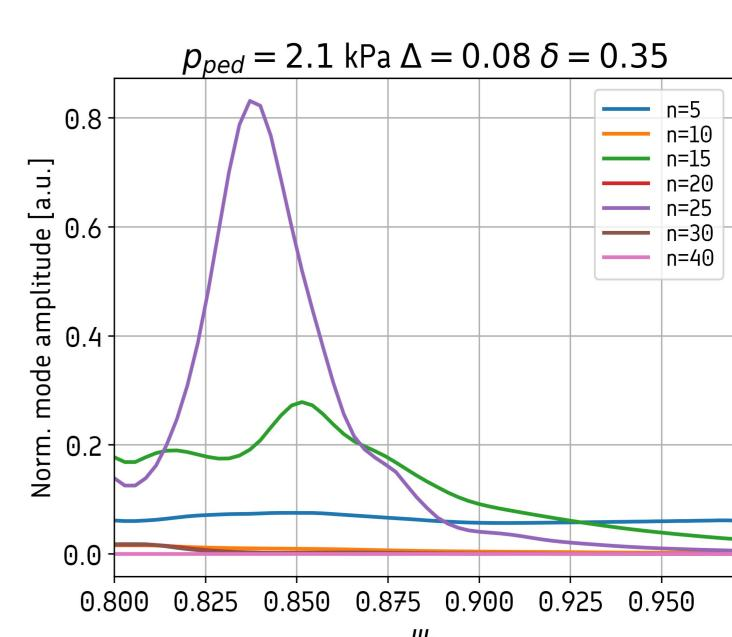
The spatial mode structure for the medium triangularity case exhibits highly notable ballooning properties, as the one mode with n=25 is dominating in the simulations. Increased values of the magnetic shear in the medium triangularity case were enough to stabilize the peeling mode branch, and it requires the additional pressure gradient to destabilize the ballooning branch of the peelingballooning mode despite the increased values of the safety factor.
