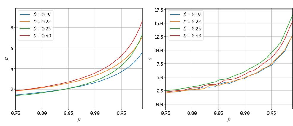
The quantitative estimations of the peeling-ballooning stability of Globus-M2 edge tokamak plasmas were carried out by the BOUT++ code [6]. The three-field model was used with the inclusion of the diamagnetic effect. The linear calculations were done with a Lundquist number of S=10<sup>8</sup>. In the poloidal direction, the 0.75-0.97 normalized flux span was covered by the 64×64 mesh.
