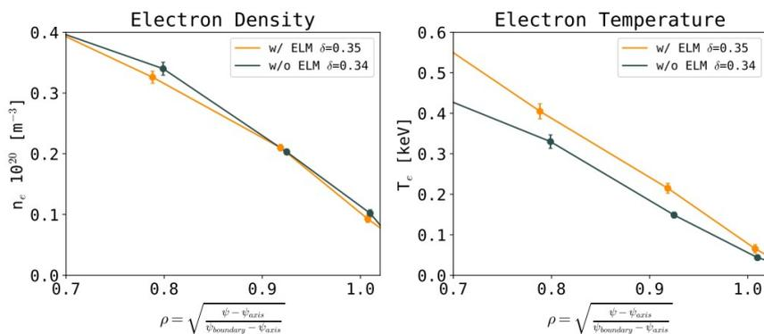
Figure 1. The electron density (left) and electron temperature (right) profiles of the Globus-M2 discharge #45936. Experimental edge data and error bars are corresponding to the Thomson scattering peripheral measurements.
