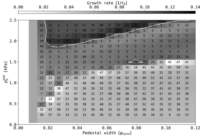
Figure 2. The stability diagram corresponding to the Globus-M2 equilibrium at  $\delta=0.34$ . The white line marks the  $0.1 \tau_A^{-1}$  boundary. Toroidal mode number of the most unstable mode is shown for each simulation.
