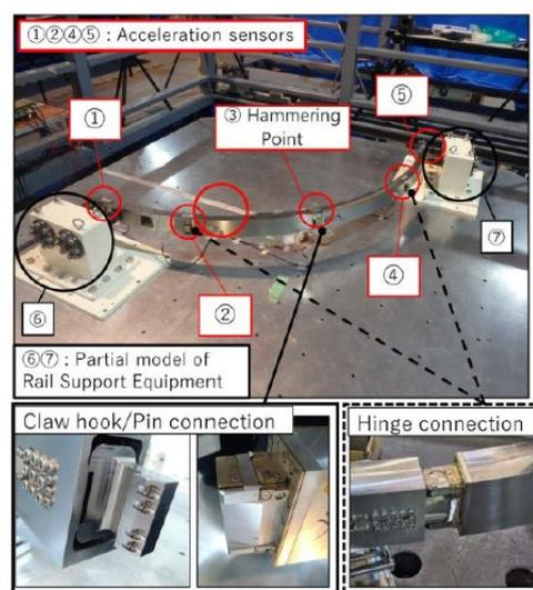
Fig. 2 Setup of the vibration tests with the scaled rail mockup[2].
