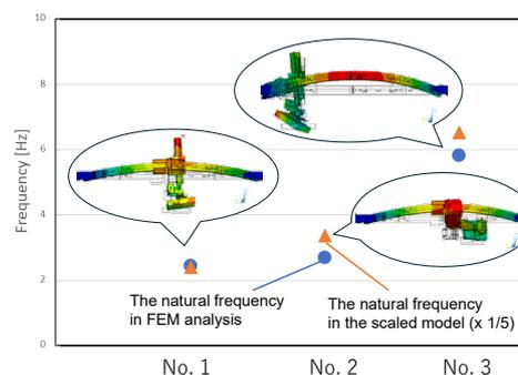
Fig. 3. Comparison of natural frequencies in vibration tests and FEM analysis in three representative postures.
