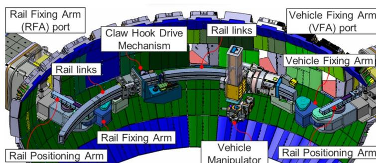
Fig. 1 Overview of the equipment involved in the In-Vessel Rail Connection process[2].
