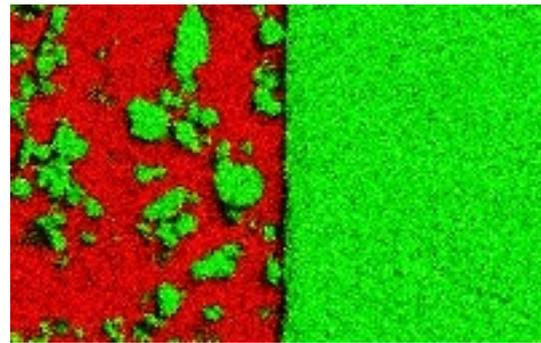
Fig. 1. SEM/EDS image at transition surface between Cu/W-interlayer (left) and bulk-W (right).
