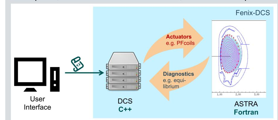
Automated Schedules: rule-based disruption avoidance, parameter scans and optimum searches in a single pulse
