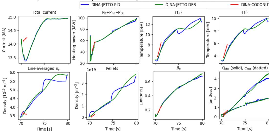
Figure 1. Time-traces of global plasma quantities in DINA-JETTO (either PID controller or default feedback controller (DFB) is used to control the line-averaged density using pellets) and DINA-COCONUT simulations (with PID) during the L-H transition phase of the 15MA/5.3T DT ITER scenario. The simulation interval of the DINA-COCONUT case is [70.5-71.3s] whereas it is [70.0-80.0s] in the DINA-JETTO cases
