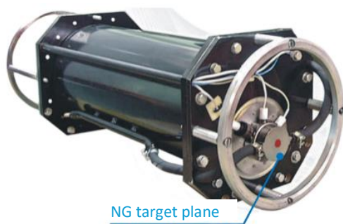
Fig.1. Irradiation unit of D-T neutron generator NG-14 with yield up to 10^{10} n/s
