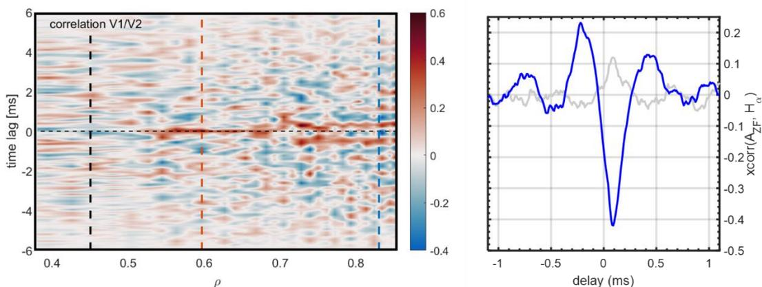
Figure 1: On the left, radial profile of the correlation between two remote Doppler reflectometer systems in W7-X, showing the ZF signature at the outer core ( $\rho \sim 0.6$ ) [1]. On the right, correlation between a TJ-II  $H_\alpha$  monitor –proxy for the particle outflux- and the global  $E_r$  oscillations, showing the modulation of particle transport by the ZF [5].
