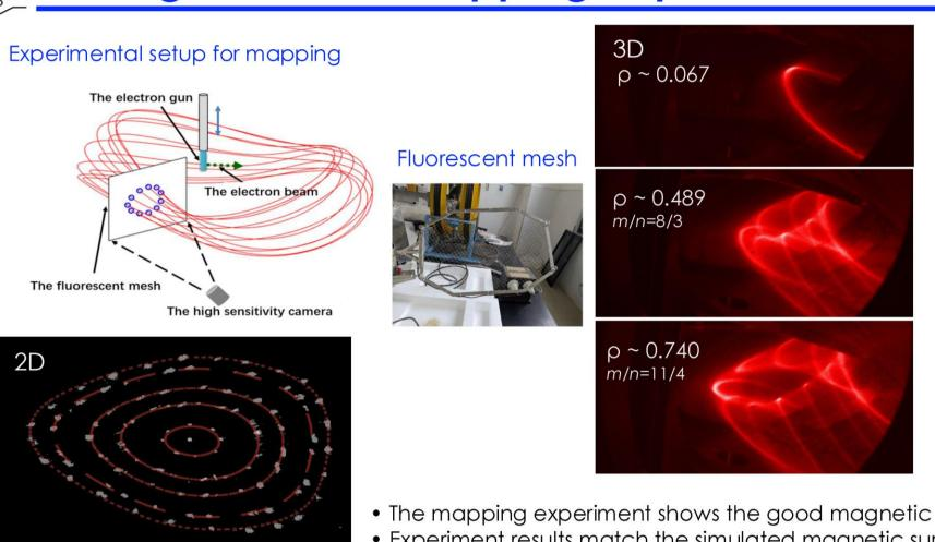
• The mapping experiment shows the good magnetic surfaces. • Experiment results match the simulated magnetic surfaces.
