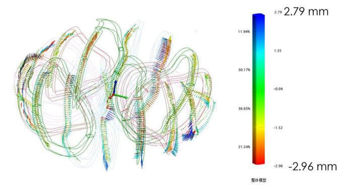
The final deviation of MC assembling is -2.96~2.79 mm.
