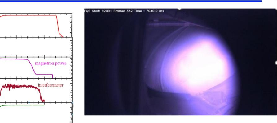
The CFQS-T plasma is produced by 2.45 GHz magnetron.
