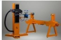
Fig. 1. Detonation spraying facility CCDS2000 with a manipulator
