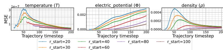
Figure 3: Long rollout error for FNO model trained on low-fidelity JOREK dataset relative to trajectory timestep. Each line is a rollout started at a different point in the trajectory (using timesteps as input prior to that point) with accumulating input error caused by the autoregressive rollout.
