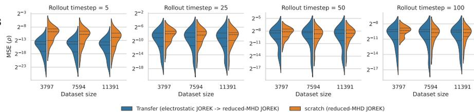
Figure 2: Comparison between model trained (orange) from scratch on the higher fidelity JOREK simulations and (blue) transferred from a lower fidelity JOREK dataset (density field) trained on different dataset sizes. Each column corresponds to a different rollout timestep, with the rollouts getting longer towards the right.
