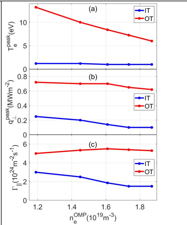
Fig.2 Peak values of the electron temperature (a), perpendicular heat flux (b), and parallel particle flux density (c) at the inner and outer targets, as a function of the separatrix plasma density at the outboard mid-plane.
