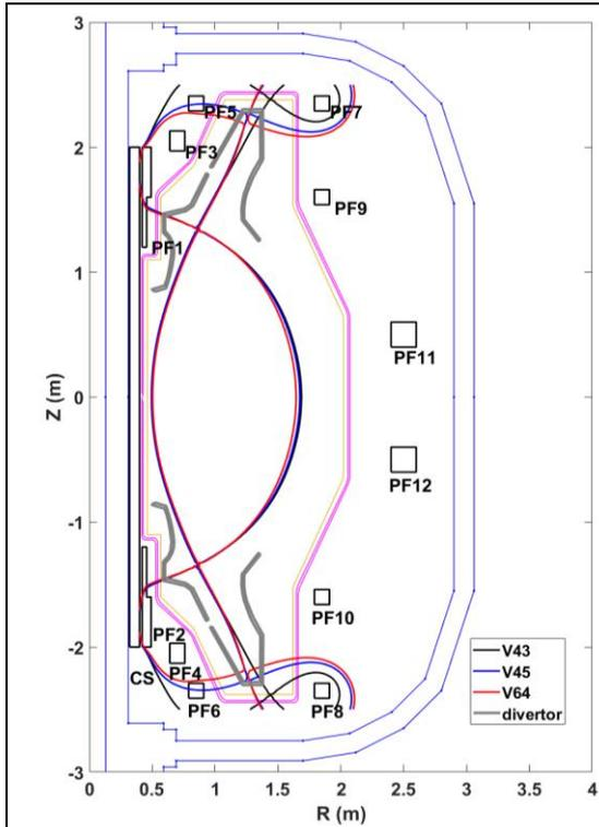
Fig.1 PF system with 12 coils; XPT equilibrium configurations with positive current PF5&PF6 ( V43 black line), without PF5&PF6 (V45 blue line) and with negative current of PF5&PF6 (V64 red line);; divertor baffle and target plate( grey line)
