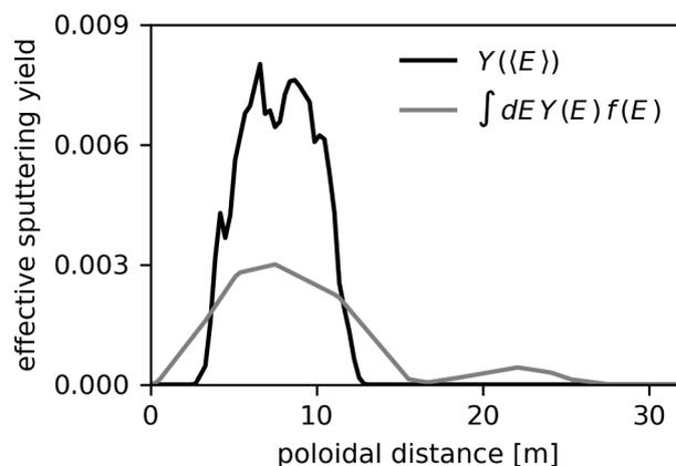
Figure 1: Effective sputtering yield obtained for the kinetic (gray) and the mono-energetic (black) energy distribution function approach.
