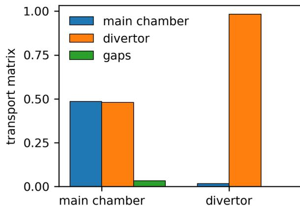
Figure 2: The figure shows the reduced transport matrix, i.e. the transport from the erosion location (x-axis) to the deposition location (y-axis).
