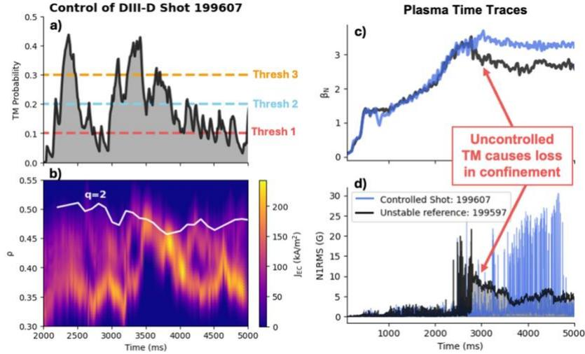
Figure 2. a) ML-based TM probability prediction with the preset threshold value for each gyrotron. b) EC current drive deposition profiles over time along with real-time  $q=2$  location used for TM suppression target. c)  $\beta_N$  time traces from a shot with feedback control compared to one without. d) NIRMS signal to where saturation of TM is clear in the uncontrolled shot.
