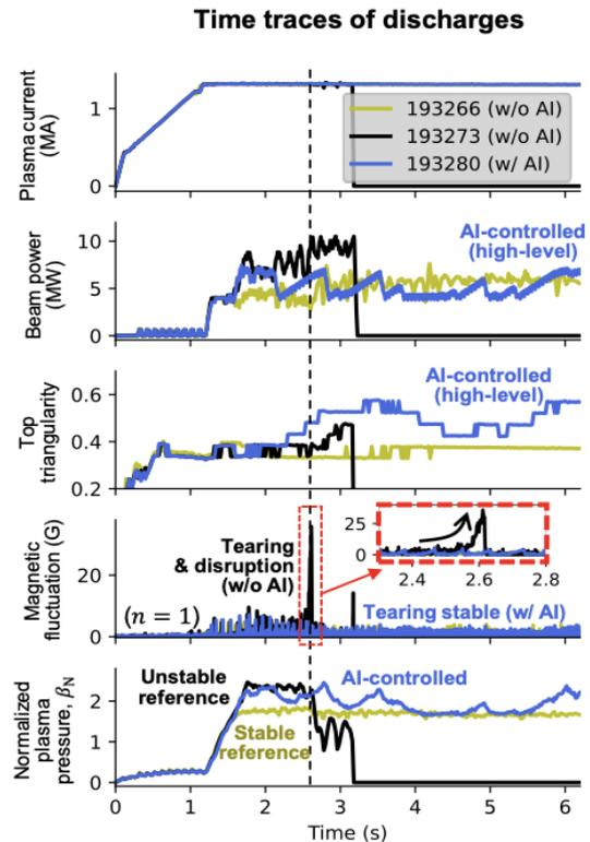
Figure 1. Time traces of various plasma parameters showing AI improvement (blue) over stable (green) and unstable (black) references. Beam power and top triangularity were the control actuators under feedback control. The magnetic fluctuations show there are no TMs in our controlled shot, and we see higher  $\beta_N$  than the stable reference shot.
