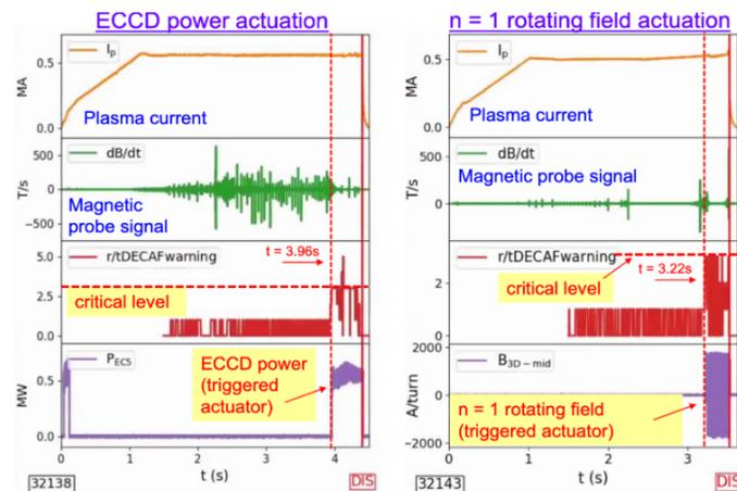
Fig. 2: Multiple actuation strategies were triggered in previous KSTAR run
