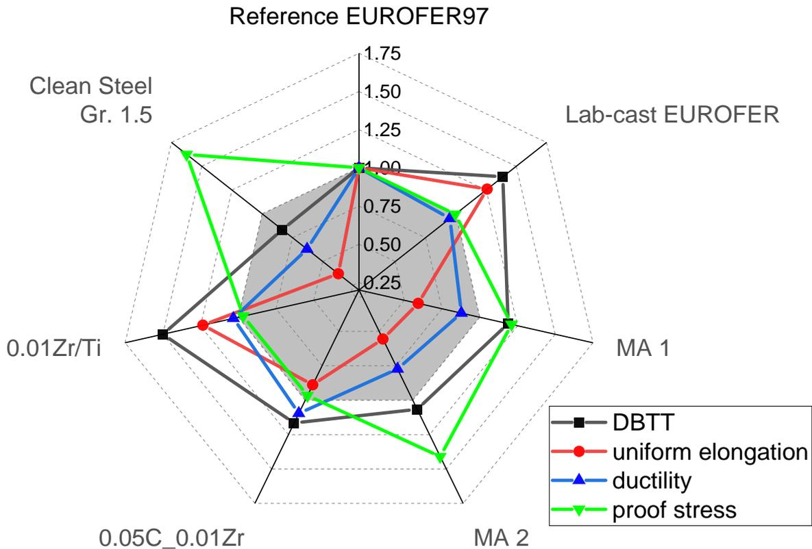
Figure 1. Quantification of improvement of the newly developed grades compared to EUROFER97 in terms of ductile to brittle transition temperature (DBTT), proof stress, uniform elongation and ductility. The displayed properties are normalized relative to the values measured in the EUROFER97 steel. Any point standing outside of the grey hexagon signifies an improvement of a corresponding property.
