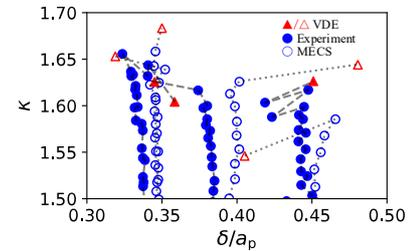
Figure 2. Comparison between  $\kappa$ -scan experiment (closed dots) and MECS simulations (open dots) regarding the relationship between  $\kappa$  and averaged gap between plasma and vacuum vessel  $\delta$  normalized by minor radius  $a_p$ .
