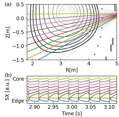
Figure 5. (a) Lines of sight of SX detector array on the contour of poloidal flux, (b) 10–1000 Hz band pass filtered soft X-ray emissions with off-axis sawtooth-like crashes.
