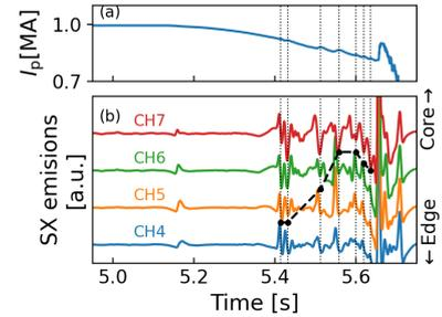
Figure 4. Typical waveforms of (a)  $I_p$  and (b) 10–100 Hz bandpass filtered line integrated SX emissions for radiative disruption. The dashed vertical lines represent the timing of  $I_p$  spikes and the black-dashed line in (b) indicated the SX spike reversal positions.
