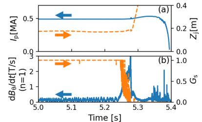
Figure 3. Typical waveforms of (a)  $I_p$  and  $Z_j$  and (b)  $n = 1$  magnetic perturbation amplitude and  $G_s$  for control failure disruption.
