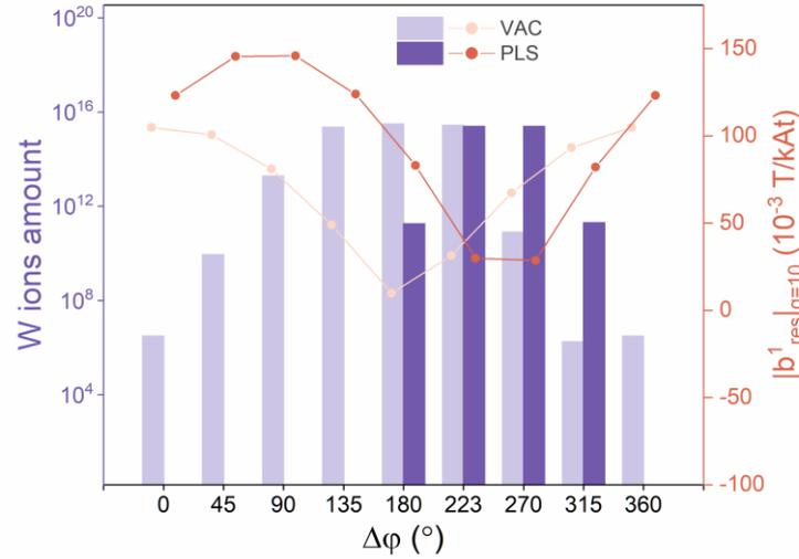
Fig 1. Comparison of integral  $W$  ions amount and  $|b^1_{res}|$  at the last rational surface ( $q=10$ ) for vacuum and plasma response field with varying coil phase difference  $\Delta\phi$  for toroidal mode number  $n = 1$  and coil amplitude  $I = 8.8kAt$ .
