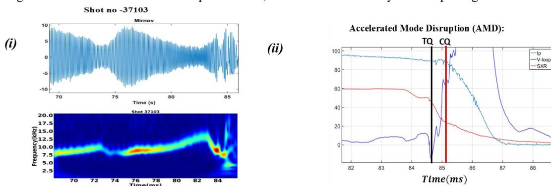
Fig. 1. (i) Time evolution of MHD mode amplitude and frequency (ii) Disruption characterized using loop voltage negative spike ( $V_{loop}$ ), thermal quench (SXR) and current quench ( $I_p$ )
