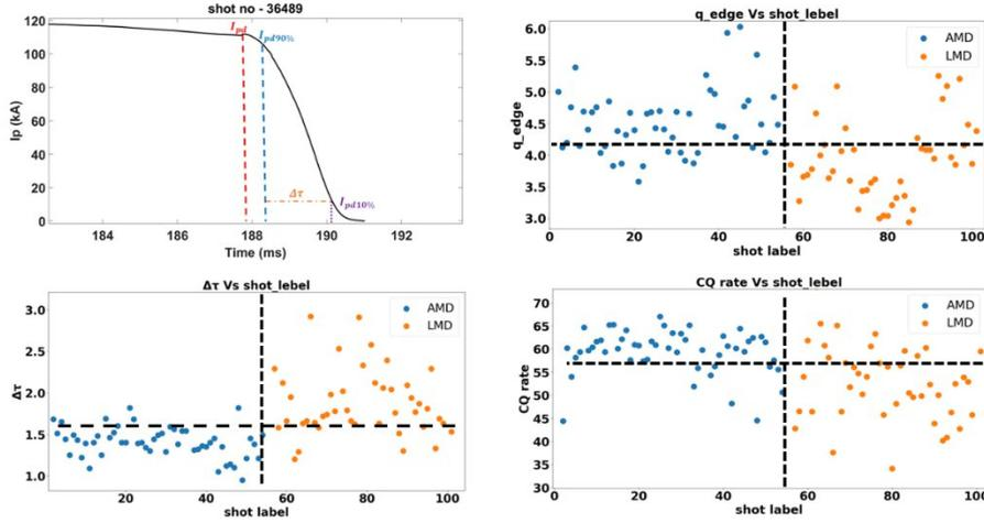
Fig. 2. (i) Current Quench characterization (ii) Statistical data of  $q_{edge}$  value for AMD and lock mode disruption (iii) Statistical data of time for current quench in AMD and lock mode disruption (iv) Statistical data of CQ rate for AMD and lock mode disruption
