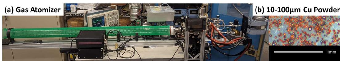
**Fig. 2.** A gas atomizer (a) produced atomized copper alloy powder particles by melting elemental mixtures within a tube furnace at 1800C that was injected into a supersonic argon atomization gas flow that breaks up the melt into fine droplets. Atomized powder diameters range from 10-100um in diameter (b).
