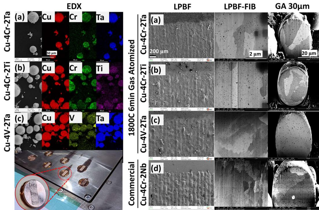
**Fig. 1.** Gas atomized powders showed consistent alloying with EDX analysis (a-c, left). L-PBF of atomized powders produced a layer of AMed material on SEM stubs inset into the build plate (bottom left). L-PBF parameters for reduced activation alloys (a-c, right) were equivalent to GRCo-42 (d). Refinement of precipitate size during L-PBF of novel alloys was similar to GRCo-42 (a-d, right).
