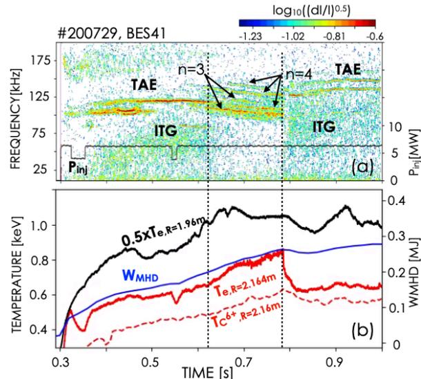
Fig. 2 Time evolution of ITG and TAE amplitudes measured by BES, along with neutral beam heating power in (a); electron and ion temperature along with the stored energy in (b).
