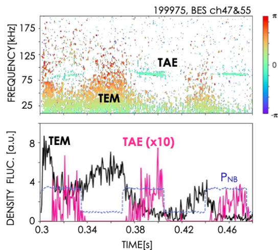
Fig. 1 (a) Time evolution of phase shift in density fluctuations between two BES channels that are separated poloidally by 1.5cm at radial location  $R=2.22m$  is shown for shot 199975 with a modulated beam of 81keV. TAE and TEM are labeled. (b) Time evolution of TEM (black curve) and TAE (red curve) amplitudes.
