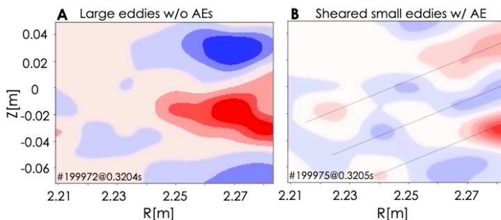
Fig. 3 Turbulent eddy images, obtained by BES system, in low voltage neutral beam of 3MW without TAE (A) and in high voltage beam of 3.3MW with TAE (B).
