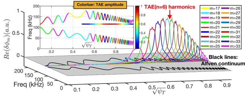
Fig. 2 Tunneling interaction between  $n=6$  TAE and Alfvén continua in DIII-D shot #159243. The TAE energy is dissipated by the kinetic Alfvén waves characterized by fine scale structures on top of each  $m$ -harmonics.
