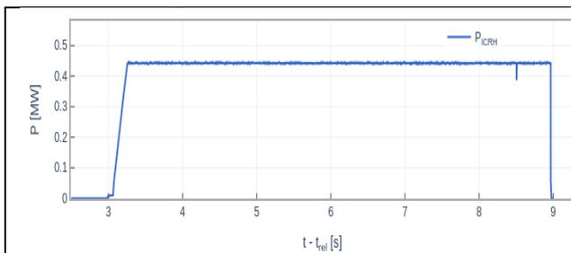
Fig.1: Example of a high power long pulse experiment (450 kW, 6s) without breakdowns at the antenna obtained with the two-strap antenna in W7-X (pulse no: 20241017.33)
