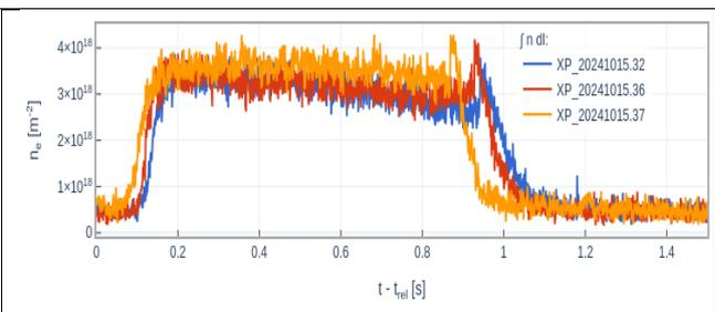
Fig.2: Line integrated plasma densities reached in plasma startup experiments (RF pulse length ~1s) with the two-strap antenna at 1.7 T and RF antenna powers between 200 kW and 400 kW.
