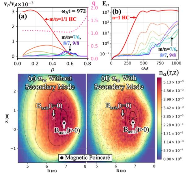
Fig. 2 (a) Radial MHD velocity profile and (b) time evolution of mode energies, highlighting the emergence of secondary modes after HC formation, with times normalized by the Alfvén frequency  $\omega_A$ . (c-d) Poloidal cross-section of alpha density after HC formation, comparing cases without and with secondary modes. Black markers indicate the magnetic Poincaré plot.
