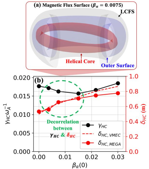
Fig.1 (a) Magnetic flux surfaces in a HC equilibrium, (b) Dependencies of the HC linear growth  $\gamma_{HC}$ , left axis, and saturated displacement  $\delta_{HC}$ , right axis, on the normalized alpha pressure  $\beta_\alpha$  in the ITER-like hybrid scenario with  $q_0/\rho_{qmin}=1.1/0.57$
