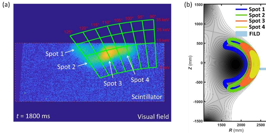
Fig. 1 A typical pattern image of the FILD during fishbone in shot 6011. The fluorescence pattern in the FILD vision (a). The unperturbed orbits of the spots in FILD vision (b).
