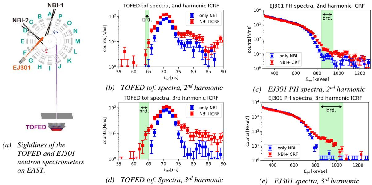
Fig. 1: Diagnostic Sightlines and Results of EJ301 Pulse Height (PH) and TOFED Time-Of-Flight (tof.) Spectra on EAST
