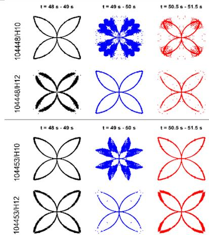
Fig. 3 The SDP plots for SXR channels H10 and H12 for the 3 selected time windows for #104448 and #104453 discharges.
