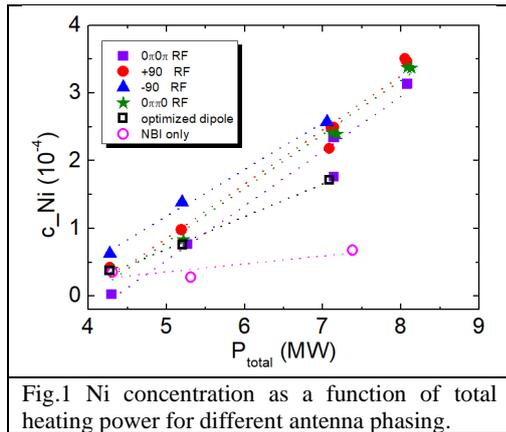
Fig.1 Ni concentration as a function of total heating power for different antenna phasing.
