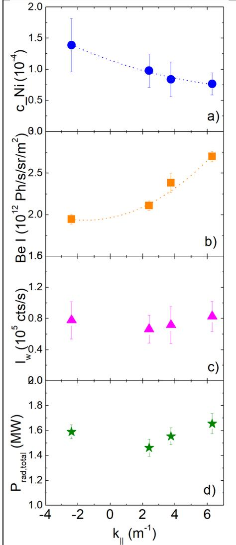
Fig.2 Ni concentration, Be I line intensity,  $I_w$  and total radiated power as a function of the parallel wave number  $k_{||}$ .
