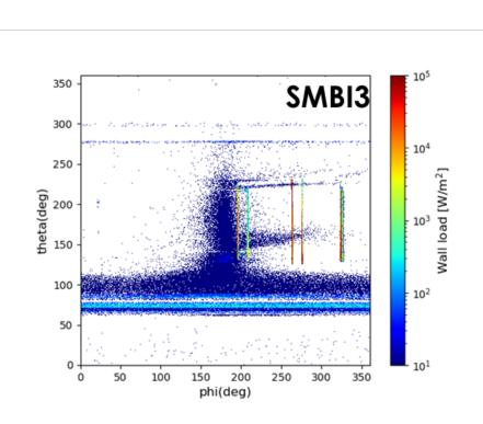
✓ The wall load on the limiter from re-ionized beam ions is significantly lower than the damage to local PFCs caused by fast neutrals
