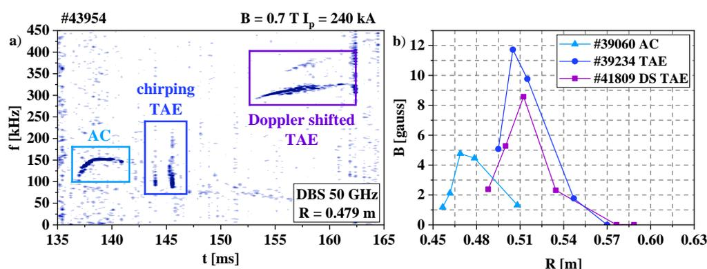
Fig. 1. a) spectrogram of phase derivative of the 50 GHz Doppler backscattering channel, b) radial profiles of AE magnetic field amplitude obtained using multi-frequency Doppler backscattering.
