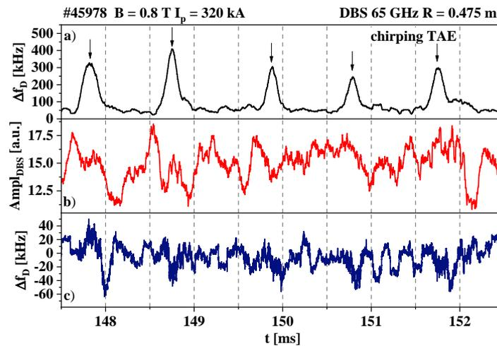
Figure 2. a) AE amplitude, b) amplitude of complex DBS signal, c) Doppler frequency shift  $\Delta f_D$  for the 65 GHz DBS channel.
