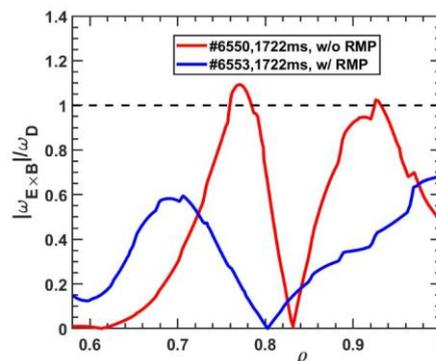
Figure 1. Turbulence suppression parameter  $|\omega_{E \times B}|/\omega_D$  with and without RMP cases.
