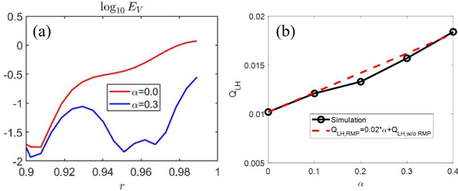
Figure 2. (a) Radial profiles of the mean square of mean flow shear before L-H transition in different  $\alpha$  (proportional to the square of the strength of magnetic perturbations) cases. (b) L-H power threshold  $Q_{LH}$  with respect to  $\alpha$ .
