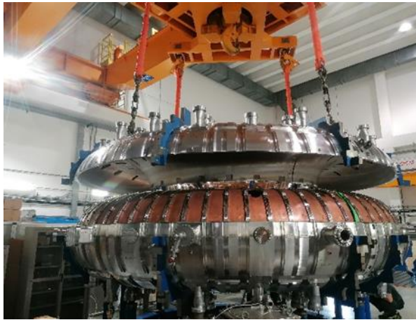
Fig. 1: closing the VTSS with the preliminary assembled PSS inside
