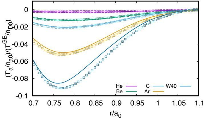
Fig. 2 Neoclassical particle fluxes of impurities ( $\text{He}^{2+}$ ,  $\text{Be}^{4+}$ ,  $\text{C}^{6+}$ ,  $\text{Ar}^{18+}$  and  $\text{W}^{40+}$ ) in the circular tokamaks with the pressure pedestal ( $R_0/L_{Ta} = 2.2$  and  $R_0/L_{na} = 5.0$ ) at the edge  $r/a_0 \approx 0.8$  obtained by GT5D (solid lines) and MI (symbols).
