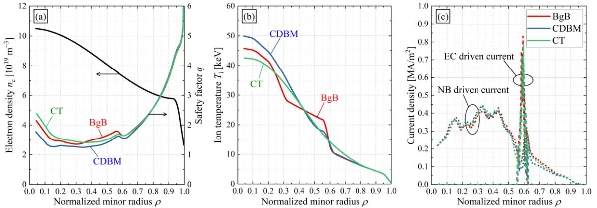
**Figure 1.** Comparison of the profiles of (a) the electron density assumed, safety factor, (b) ion temperature, and (c) NB- and EC- driven current densities obtained from the GOTRESS+ simulations between the cases using the BgB, CDBM, and CT models.
