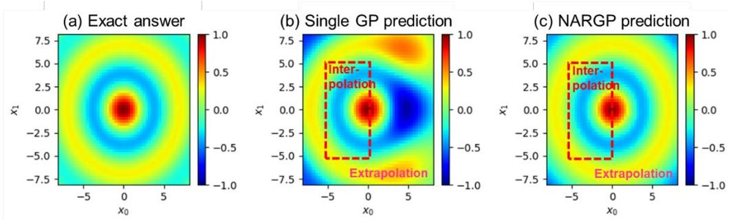
Figure 1. Extrapolative prediction for a test function. (a) The two-dimensional test function  $f_h(x_0, x_1)$ . (b) Single GP prediction using only the test function data at the area surrounded by a red dashed square. (c) NARGP prediction using the high-fidelity and low-fidelity test function data.
