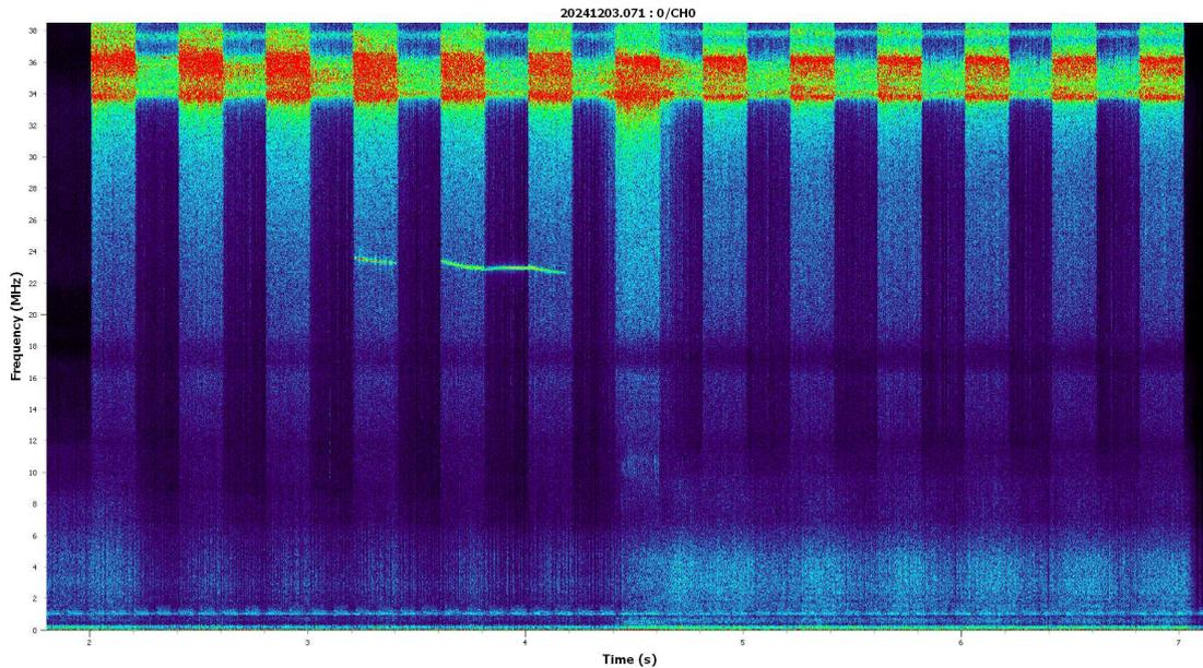
Figure 1. An example of ICE spectrum measured with the ICRF antenna in discharge 20241203.71, demonstrating the low-frequency activity at around 20 MHz and a broadband ICE activity at the fundamental harmonic of ICE at around 35 MHz.
