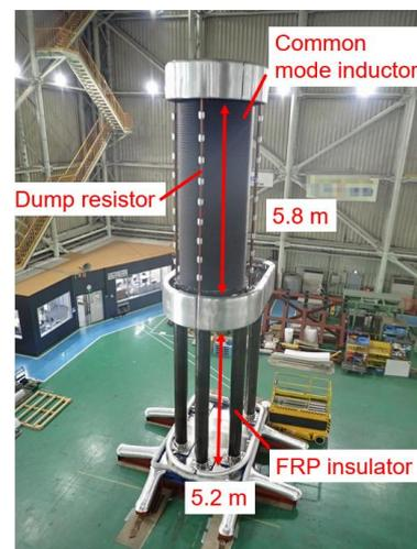
Fig. 3. Common mode filter for -1 MV insulating transformer.
