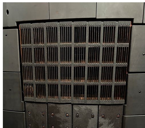
Figure 1. The HFS LHCD launcher installed on the DIII-D tokamak. The launcher includes 8 modules arranged toroidally, which are each fed by individual waveguides capable of transmitting 200 kW.
