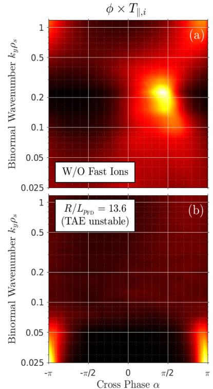
**Fig. 1:** Simulated cross-phase between electrostatic potential and parallel ion temperature fluctuations without fast ions (a) and with unstable TAE (b).
