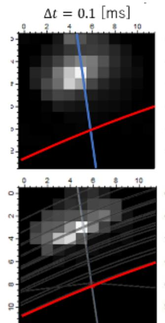
Fig. 1 2D images of the emission intensity (a) and plasmoid density (b) at the maximum emission intensity ( $t = 0.1$  ms) of the pellet ablation cloud, observed from the upper port. The pixel resolution is 12 mm per pitch. The red line indicates the magnetic axis. [shot#82554 ECH+NBI] [4].
