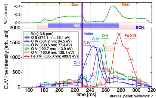
Fig. 3 Temporal evolution of the stored energy ( $W_p$ ) and the EUV line spectra, indicated by the wavelength and ionization energy.
