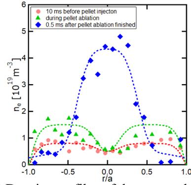
Fig. 2 Density profiles of the target plasma before pellet injection (-10 ms), during the pellet ablation (0.1 ms) and immediately after the ablation (0.5 ms from the  $H_{\alpha}$  trigger ON) [shot#79541-79546 ECH+NBI] [5].
