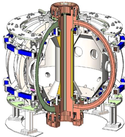
Figure 1. Preliminary design of the electromagnetic system and the vacuum vessel of the Globus-3 tokamak
