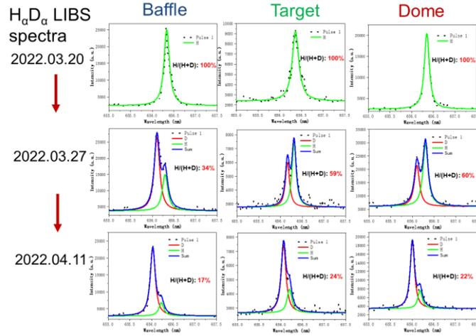
Fig. 2. The LIBS spectra of  $H_{\alpha}$  and  $D_{\beta}$  on the surface of the divertor after wall conditioning with different poloidal positions
