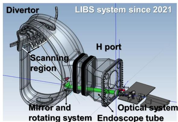
Fig. 1. The schematic of endoscope LIBS system for upper W-divertor in EAST
