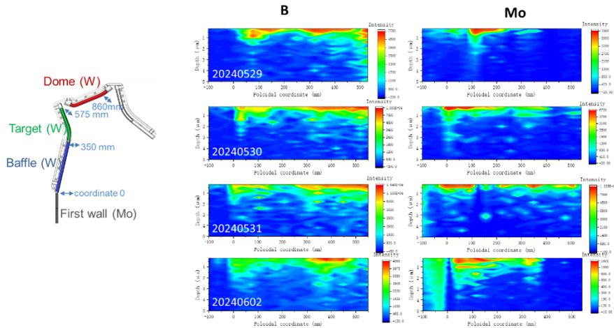
Fig. 3. The cross-section distributions of B and Mo on the upper divertor in EAST
