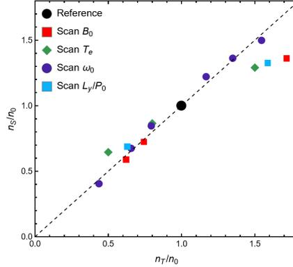
Figure 2. Comparison between density limit  $n_s$  from simulation results and  $n_T$  from the scaling relation, Eq. (1).
