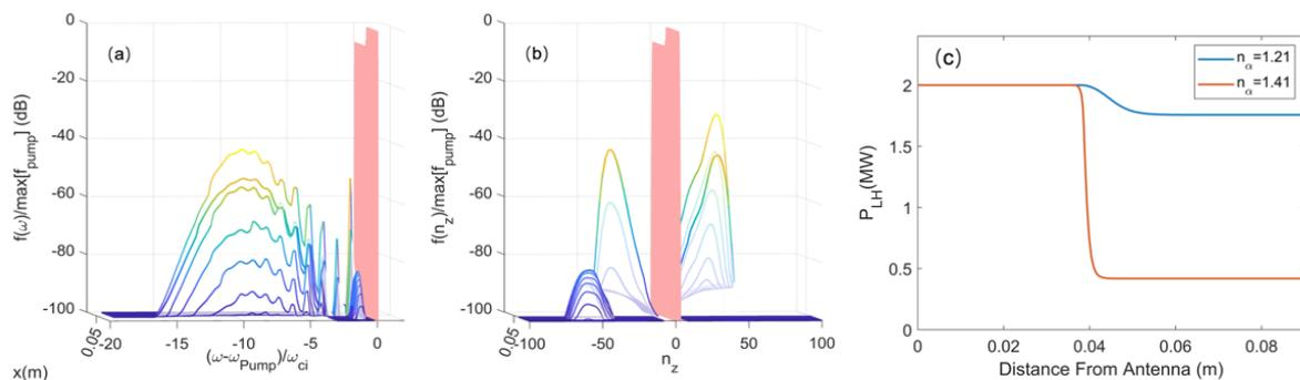
Figure 1. Evolution of LHW frequency spectrum (a) and parallel wavenumber spectrum (b) at  $n_\alpha = 1.41$ , where  $n_\alpha$  is the multiply factor for JET-like reference SOL density profile, and evolution of LHW pump power for  $n_\alpha = 1.21$  and 1.41 (c).
