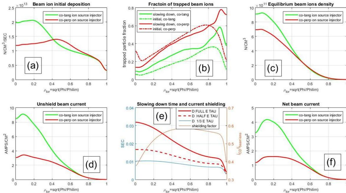
Fig.2 Analysis of NBCD details for co-tang and co-perp downward steered injectors, (a) initial deposition profiles, (b) trapped particle fraction profiles of initial and slowing down beam ions, (c) steady state beam ion density, (d) flux averaged unshielded beam ion current, (e) slowing down times of three beam energy components and shielding factor, (f) net beam current with TRANSP/NUBEAM shielding current calculations.
