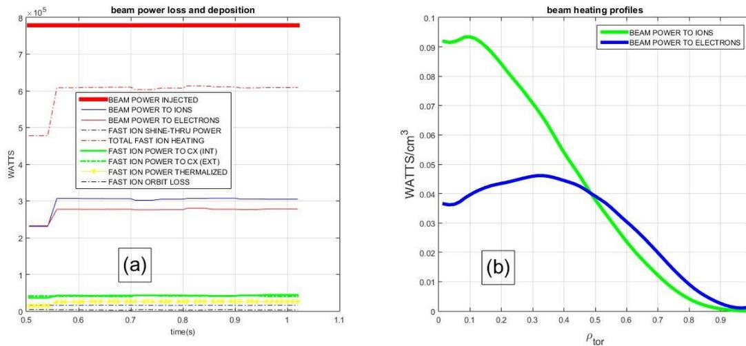
Fig.1 (a) beam power deposition and loss terms during discharge, (b) beam heating profiles.
