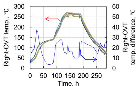
Figure 2. Temperature history and its difference of Right-OVT prototype during heating.
