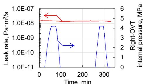
Figure 3. Leak rate during pressurization of Right-OVT prototype.
