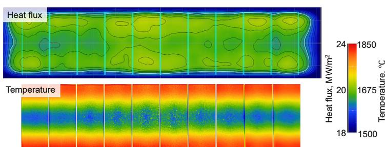
Figure 1. Profiles of heat flux and temperature during heat load at 20 MW/m<sup>2</sup>.
