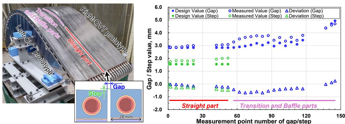
Figure 4. Measurement result of gaps and steps between Left- and Right-OVT prototypes. (The OVT has a shape that widens from the straight part to the baffle part, and the width of the W block varies from 28.0 mm to 30.3 mm. Because the variety of monoblock widths is limited, the gap design value does not change monotonically.)
