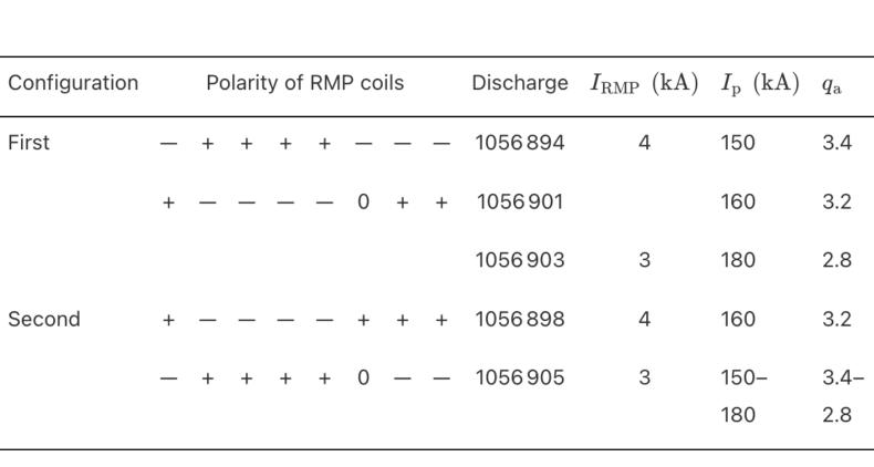
RMP coil setup and plasma parameters implemented in the experiment.
