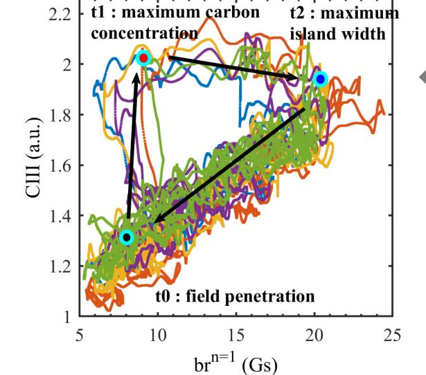
The relation between CIII and b<sub>r</sub> during five collapses Overview of the discharge #1077700
