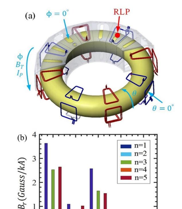
2D Fourier (m, n) spectrum of the radial magnetic field generated by RMP coils at the plasma edge
