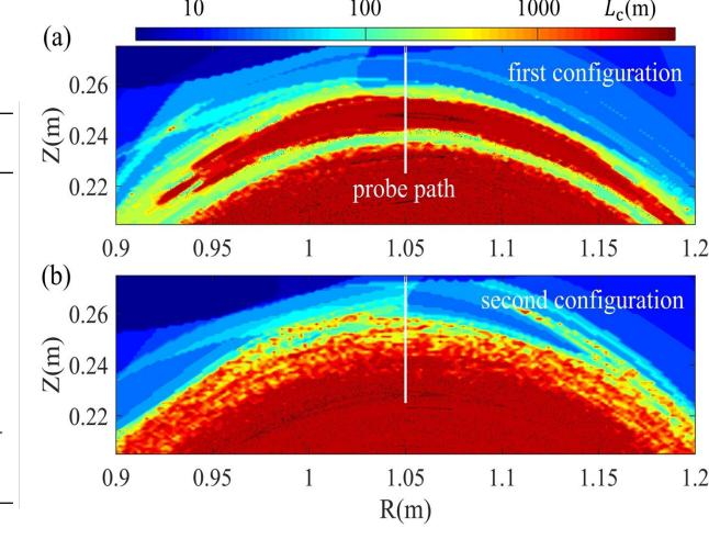
The connection length  $L_c(R, Z)$  for two different RMP configurations
