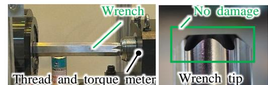
Fig.5 Torquing test and result
