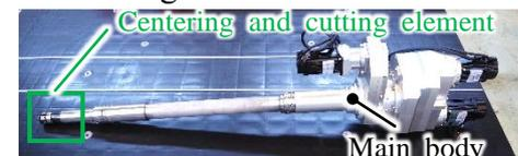
Fig.4 Prototyped Cutting Tool
