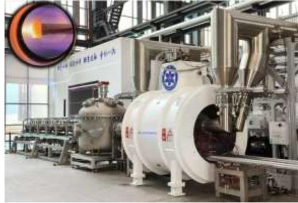
Figure 1. The SWORD facility and its target exposed to high flux He plasma.
