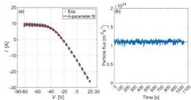
Figure 2. (a)  $I$ - $V$  curve and the corresponding fit using the four-parameter model. (b) Continuous particle flux measurement at a fixed target bias voltage of  $-50 \text{ V}$ .
