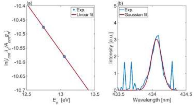
Figure 3 (a)  $T_e$  determined by the Boltzmann method, and (b)  $n_e$  determined by the Stark broadening effect.
